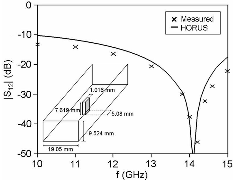
Fig. 2. Ridge waveguide measured in [18]. HORUS used 3rd order nodal elements. The divergence term of (8) was removed from the elements in contact with the edges of the ridge.
