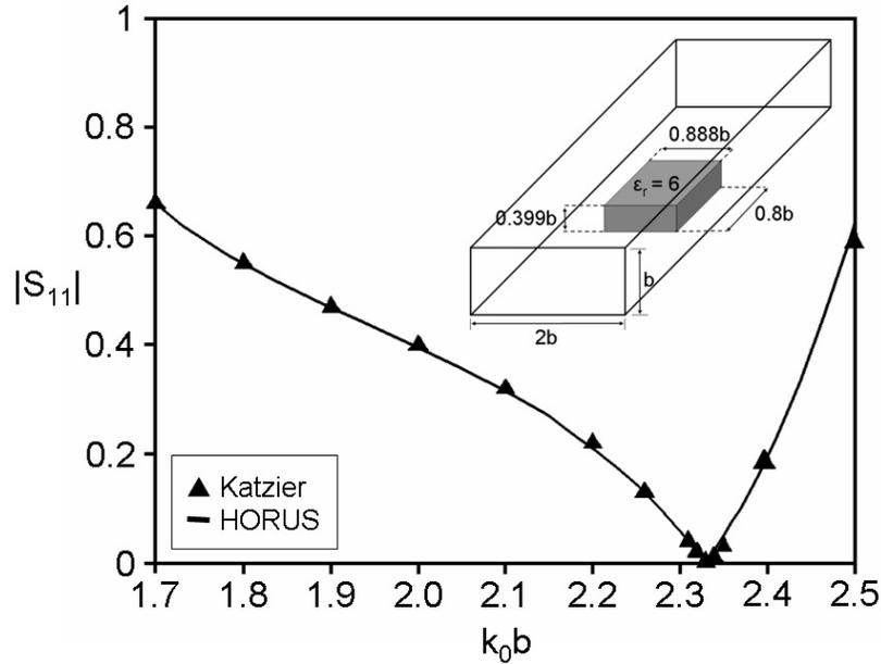
Fig. 3. Method in [19]. HORUS used 3rd order nodal elements. The divergence term of (8) was removed from the elements in contact with the edges of the dielectric.
