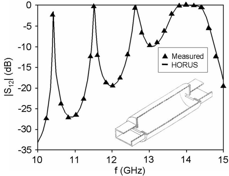
Fig. 1. Circular cavity filter measured in [17]. HORUS used 3rd order nodal elements. The divergence term of (8) was removed from the elements in contact with the edges of the coupling slots.
