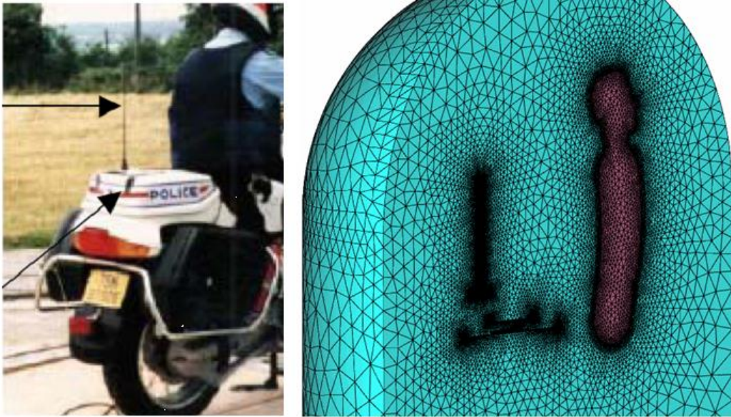
Figure 10: PROCOM MU9-XP4 antenna installed in a motorbike. Left: real geometry. Right: FEM mesh by GiD [28] used for HORUS simulations. The mesh is composed of tetrahedral 2nd order nodal elements.
